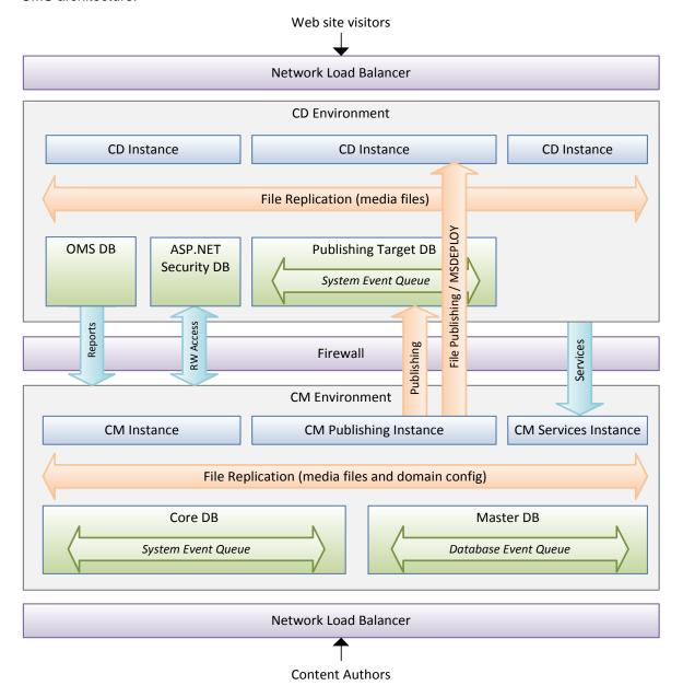
The lower section illustrates the CM environment. The rightmost CM server is configured to host the services that the CD servers use to communicate across the firewall. The upper section illustrates the CD environment. The CD instances use the service layer to access the CM environment and manage orders, product stock, and price information.
